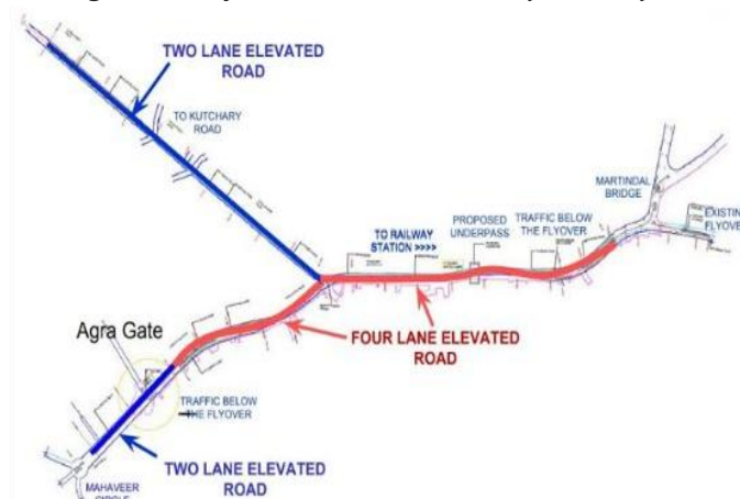
Fig. 4: Outlay of Elevated Road Project in Ajmer
